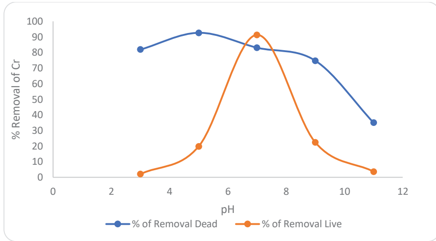
Fig. 2: Effect of pH on biosorption of chromium by dead and live biomass.
